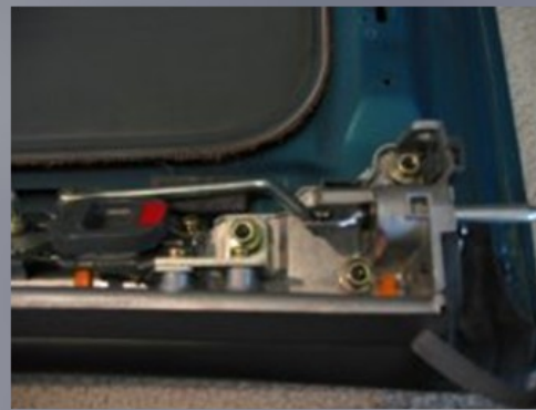
Remove the 3 10mm nuts from front of each rail
