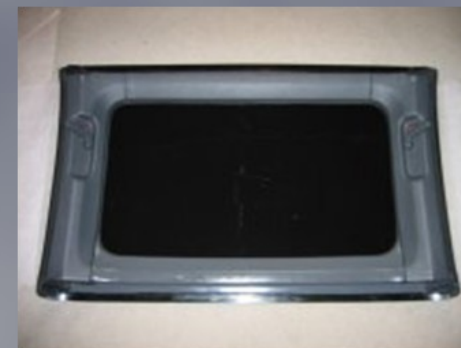
Install the plastic garnish on the new roof - note, the front-center piece didn't snap in place until the metal tabs were bent/expanded so they could catch
